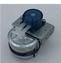
The 100CPT series, micro range of peristaltic pumps offer a low cost, compact & reliable means of dosing a wide range of liquids. They are available in various configurations of tubing type & size giving flow rates of between 0.08 & 0.26 ml/rev. The pump head is designed to be disposable but is assembled using two screws enabling dis-assembly & re-assembly for tube changing if required.
