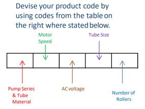
102CPT-015-230-016/4 Example product code for 100CPT series pump head fitted with Viton® tubing, 15 RPM, 230v AC, 1.6mm ID tubing & 4 rollers
