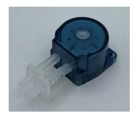
The 100CPT series, micro range of peristaltic pumps offer a low cost, compact & reliable means of dosing a wide range of liquids. They are available in various configurations of tubing type & size giving flow rates of between 0.08 & 0.26 ml/rev. The product is designed to be disposable but each pump head is assembled using two screws enabling dis-assembly & re-assembly for tube changing if required.
