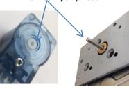
4. Push pump head fully down shaft, rotate to align screw holes and fit mounting screws (do not over-tighten)
