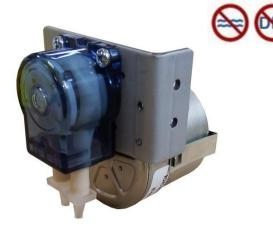
The 100 series, micro range of peristaltic pumps offer a low cost, compact & reliable means of dosing a wide range of liquids. They are available in various configurations of tubing type & size giving flow rates of between 0.016 & 0.26 ml/rev.
