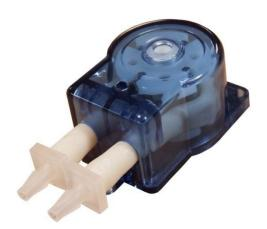
The 100 series, micro range of peristaltic pumps offer a low cost, compact & reliable means of dosing a wide range of liquids. They are available in various configurations of tubing type & size giving flow rates of between 0.016 & 0.26 ml/rev. The product is designed to be disposable but each pump head is assembled using a single screw enabling dis-assembly & re-assembly for tube changing if required.
