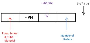
102-PH-016/4-4mm Example product code for 100 series pump head fitted with Viton® tubing, 1.6mm ID tubing, 4 rollers suitable for 4mm D shaft
