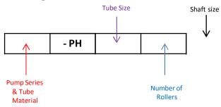
102-PH-016/4-4mm Example product code for 100 series pump head fitted with Viton® tubing , 1.6mm ID tubing, 4 rollers suitable for 4mm D shaft
