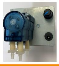
The micro range of 100 series stacked stepper motor driven pump offer a low cost, reliable means of dosing a wide variety of fluid. The pump is capable of pumping 2 different fluids in various ratios by using different tube materials/sizes on each pump head. They are available in various configurations such as: 2 or 4 roller, multiple tube materials and sizes giving flow rates between 0.0025 and 39ml per minute per pump head.
