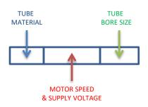
For example: A CM pump with 3mm bore silicone tube, 70 rpm 230v AC would be 200-070-230-030CM.
