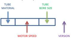
For example: A Oneshot pump with 5mm bore silicone tube, 140 rpm dosing version would be OS-200-140-050.
