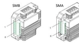
H/L must be connected to 0v for 40 & 150 rpm speed ranges. ENA, On/Off & Direction connections are optional. Pump will run clockwise once supply is connected remove to stop or alternatively connect 0v to ENA this will stop motor. Connecting 0v to ON/OFF will also stop the motor but it is a powered stop/hold so motor will remain powered all the time causing additional heat generation.
