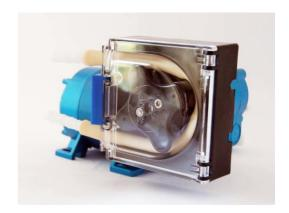
The 4000 is a high performance and versatile peristaltic pump. The hinged lid forms an integral part of the pump construction, and releasing the lid catch facilitates tubing replacement. The lid can also be removed completely for tube replacement in confined spaces. Options available for this unit include a choice of tube material and size & motor speed.
