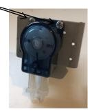
Carefully open the pump head from the base and remove back plate
