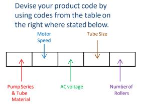
202-030-230-016/3 Example product code for 200 series pump head fitted with Viton® tubing , 30 RPM, 230v AC, motor, 1.6mm ID tubing & 3 rollers
