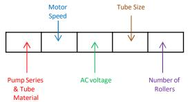
202-030-230-016/3 Example product code for 200 series pump head fitted with Viton® tubing, 30 RPM, 230v AC, motor,1.6mm ID tubing & 3 rollers
