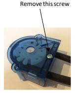
Squeeze tubes together and lift out rotor. If tube is fitted with blue "C" clips leave in place on tube. Rotate the rotor complete with tube so the other drive size is towards you.
