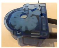
To refit the pump head first carefully locate "D" on motor shaft into the "D" in the rotor. Rotate pump head until mounting holes line up with holes in bracket. Remove pump & place mounting screws through pump head. Fit rubber washer on screw threads so that they will end up between pump head & bracket. Refit pump head and do up screws carefully. Screws must tightened sufficiently to partially compress rubber washer not completely flatten them.
